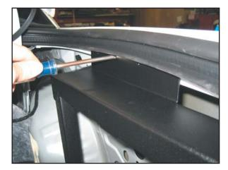
Attach top frame with three (3) - 10/32" x 1/2" machine screws and keps nuts.
